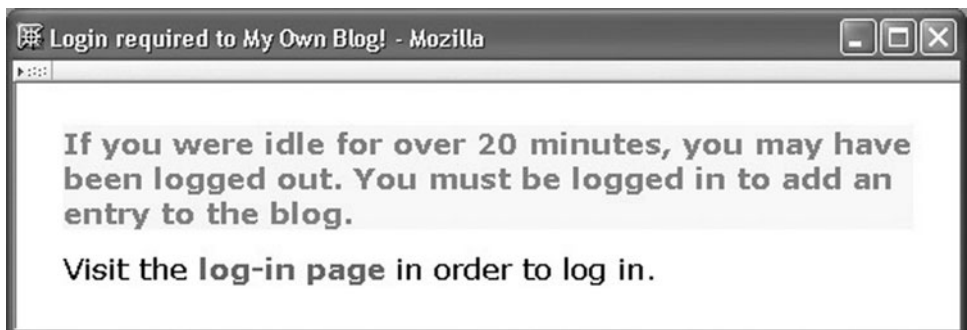
FIGURE 6.38 Page displayed if a POST request is sent to the AddOrPreview servlet and the user is not currently logged in.
