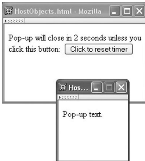
FIGURE 5.27 Pop-up window displayed in front of initial browser window containing HostObjects.html document.
