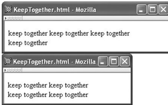
FIGURE 2.10 Two browser windows of different widths displaying an HTML file using the &nbsp; reference.
